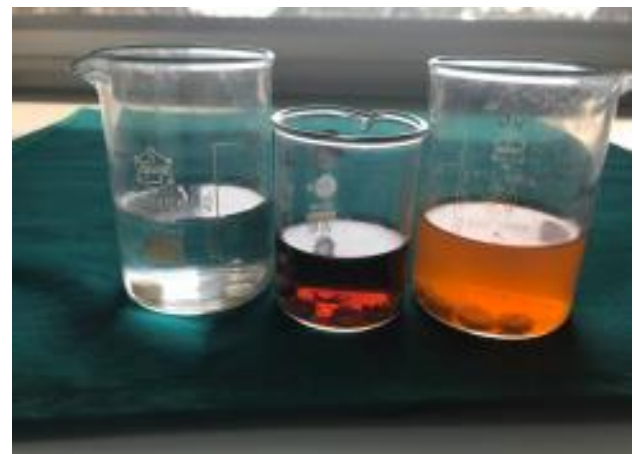
Figure 3: Samples are immersed in fizzy drinks (orange colour-miranda; brownish red colour-pepsi) and distilled water (transparent) which are contained in a glass beaker
