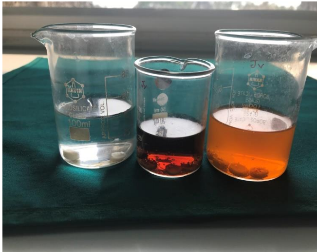
Figure 3: Samples are immersed in fizzy drinks (orange colour-miranda; brownish red colour-pepsi) and distilled water (transparent) which are contained in a glass beaker.
